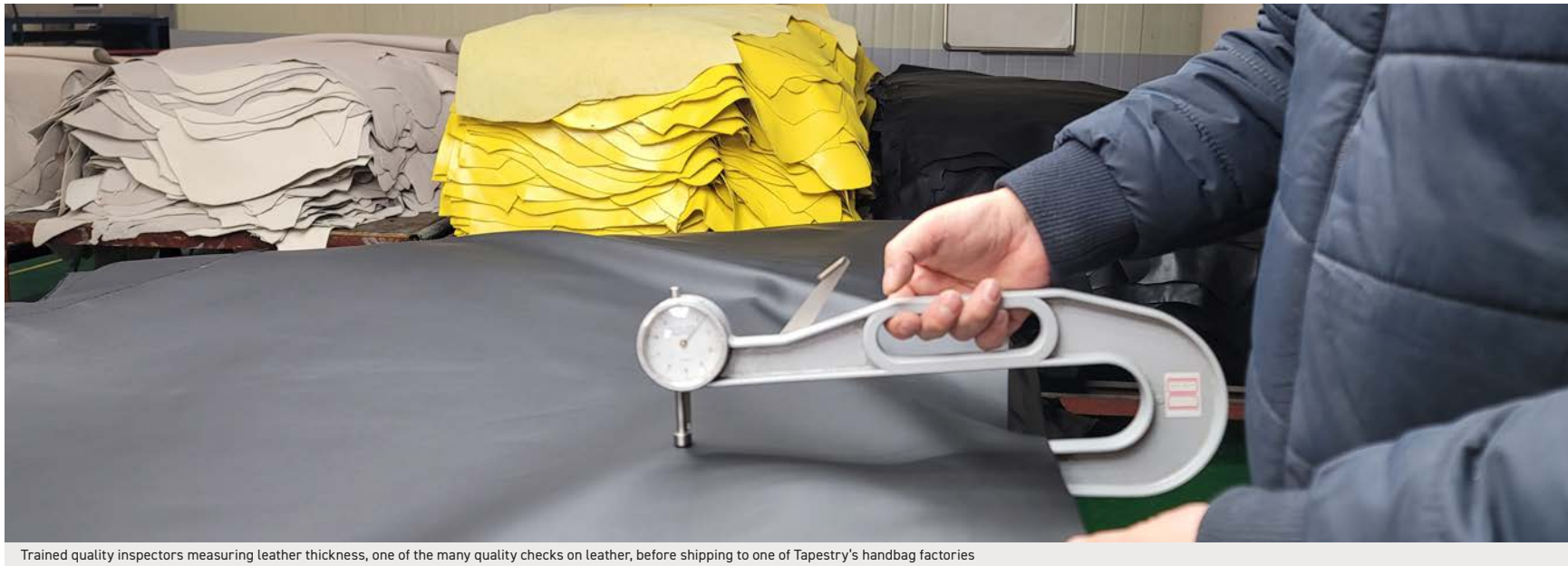
Trained quality inspectors measuring leather thickness, one of the many quality checks on leather, before shipping to one of Tapestry’s handbag factories
